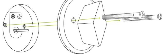
First you have to remove the existing thumb turn on the inside of the door. (On some doors it can be helpful to put a piece of tape across the lock on the outside of the door to prevent it from falling when the screws are removed).
