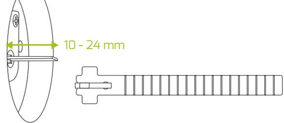
Most doors have tailpieces that extends 10 - 24 mm from the doorplate. They will fit the Danalock without need for any adjustments to their length! If the tailpiece is less than 10 mm long from the door surface, an extra tailpiece can be found in the Danalock box. (see the 2 next illustrations)
